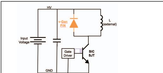
**Fig. 3. DPTC used to evaluate the switching characteristics of v-GaN diode as well as SiC SBD and conventional Si diode under loaded switching conditions**
