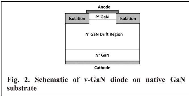
the minority carriers injected across the junction. When conducting current, the diode is flooded with minority carriers, which causes current to flow across the junction. When switching from conducting to blocking, the minority carriers present in the depletion region must be swept out via recombination, which is manifested as a reverse current [3, 16]. Although junction capacitance also contributes, for Si devices this minority-carrier recombination limits the reverse recovery time.
