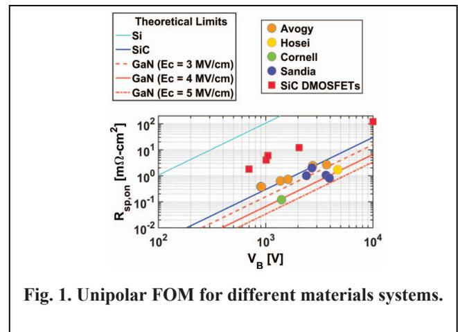
Fig. 1. Unipolar FOM for different materials systems.
