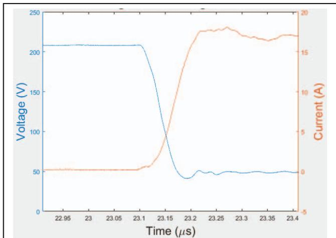
**Fig. 6. GaN PiN diode blocking-to-conducting transition voltage and current traces, at  $V_{in} = 200$  V.**
