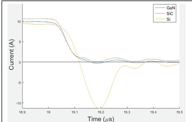
**Fig. 7. Conducting-to-blocking for v-GaN PiN diodes, SiC Schottky SBDs, and Si diodes. The SBD and v-GaN diodes show negligible reverse recovery while the Si diode shows a distinct reverse recovery region.**
